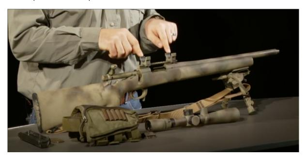
During firing, inertia will cause the rings to move forward relative to the rifle and by having them at their forward limit already, you'll reduce their possibility of them moving once installed.
