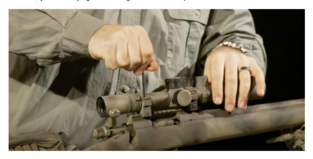
Tighten the rings around the scope by turning the screws in an X pattern (similar to changing a wheel on a car) while ensuring that the gap on each side of the rings is similar.
